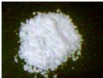
Figure 1. A sample from struvite formed from the synthetically prepared wastewater in this study
